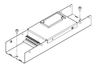
2) Terminal covers support 1/2" trade size conduit fittings. To meet UL requirements conduit or armoured cable must be used for power input cables.
