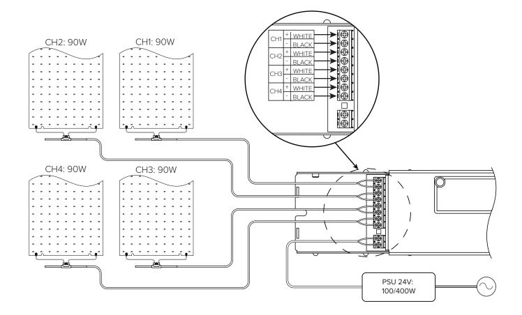
CONTROLS INPUTS: 0/1 - 10V STATIC COLOR TEMPERATURE (SCT)
