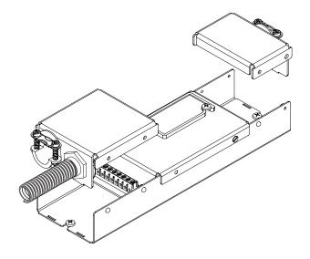
4) Snap covers in position and secure with provided fasteners.
